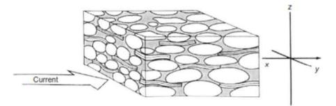
FIGURE 6.22 Block diagram of sand showing layered fabric with grains oriented parallel to current. Generally,  $K_x > K_y > K_z$ .
