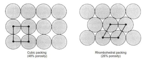
FIGURE 6.21 The loosest and tightest theoretical packings for spheres of uniform diameter.
