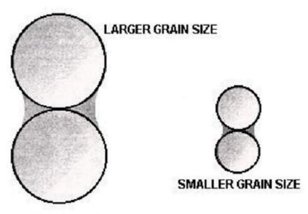
Figure 31 Grain size effects on capillary pressure and pore throat diameters.
