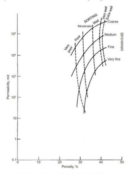
FIGURE 6.20 Graph of porosity against permeability showing their relationship with grain size and sorting for uncemented sands. After Beard and Weyl (1973), Nagtegaal (1978).
