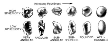
FIGURE 6.19 Sand grains showing the difference between shape and sphericity.
